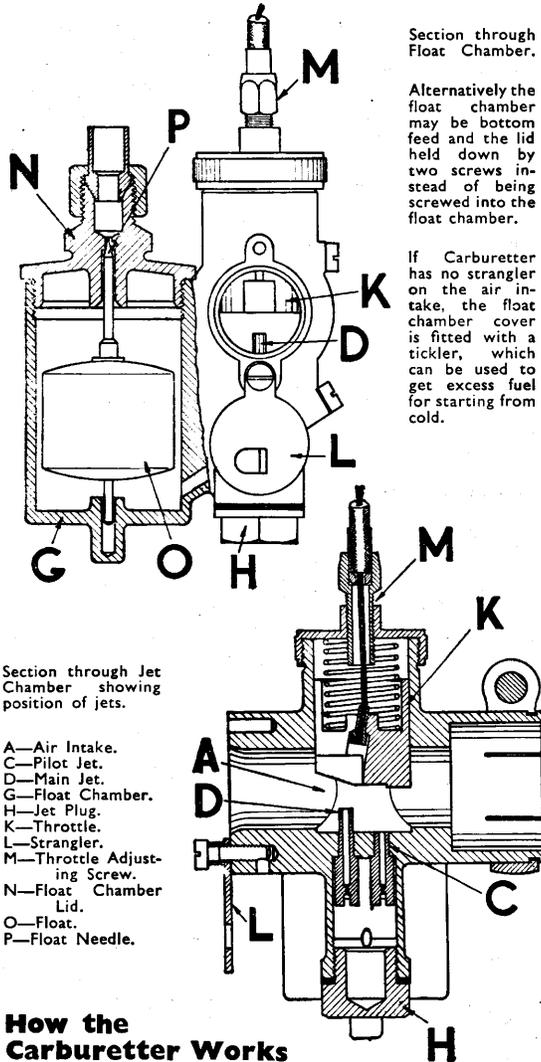
Section through Float Chamber.
