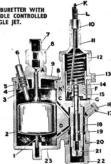
This sectioned diagram is taken through the centre of the mixing chamber and float chamber, showing the float and jet and throttle mechanism. The float and needle are shown as one piece as for types 259 and 261, but in type 223 the float needle (1) is separate from the float (2), but is attached thereto by a spring bow fastened to the float at the place marked (E). The cable (K) and its anchoring (K1) are diagrammatic as in practice the cable anchoring is in front of the jet.
